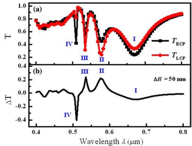
**Fig. 2.** (a) Simulated transmission spectra of LCP and RCP light for the chiral heterodimers. (b) Differences of transmittance spectra of heterodimers with  $\Delta H = 50 \text{ nm}$  between LCP light and RCP light.
