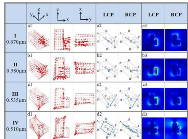
**Fig. 3.** (a1–d1) Distributions of surface current density of the chiral heterodimers, (a2–d2) detail path of resonant modes, and (a3–d3) steady-state electric field distributions of the chiral heterodimers under the illumination of RCP and LCP.
